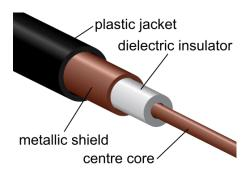
Figure 1-3 Coaxial cable
