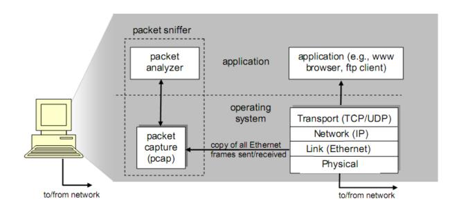
Figure 10-1 Packet Sniffer Structure
